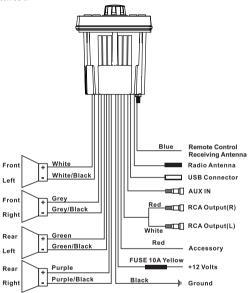
Tip: When a suitable ground wire is not present in the vehicle wiring harness. Connect the black ground wire to the vehicle chassis.
